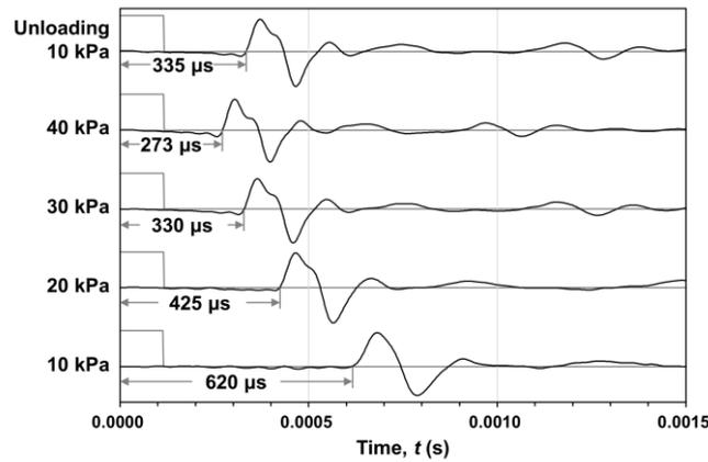
Fig. 2. Example of interpretation of travel time from shear waves.
