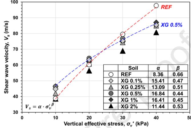
Fig. 6. Correlation between the vertical effective stress and the shear wave velocity from the consolidation test (after loading).
