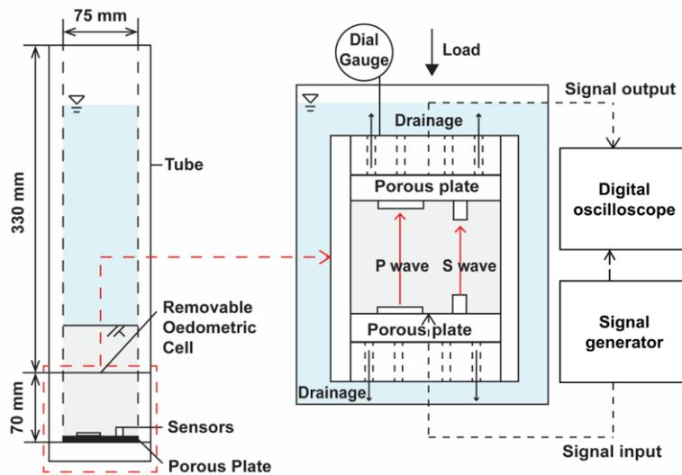
**Fig. 1.** Experimental setup: Sedimentation tube with a removable oedometric cell (adopted from Chang and Cho (2010)).
