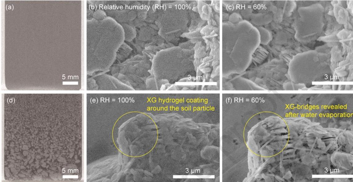
**Fig. 9.** Visual analysis of kaolinite suspensions: (a) X-ray CT scan of uniform kaolinite suspension (in grey) without XG treatment, ESEM images of untreated kaolinite at the relative humidities of (b) 100% and (c) 60%, (d) X-ray CT scan of XG-kaolinite aggregates (in grey) in deionized water (in black), and ESEM images of XG-treated kaolinite at the relative humidities of (e) 100% and (f) 60%.
