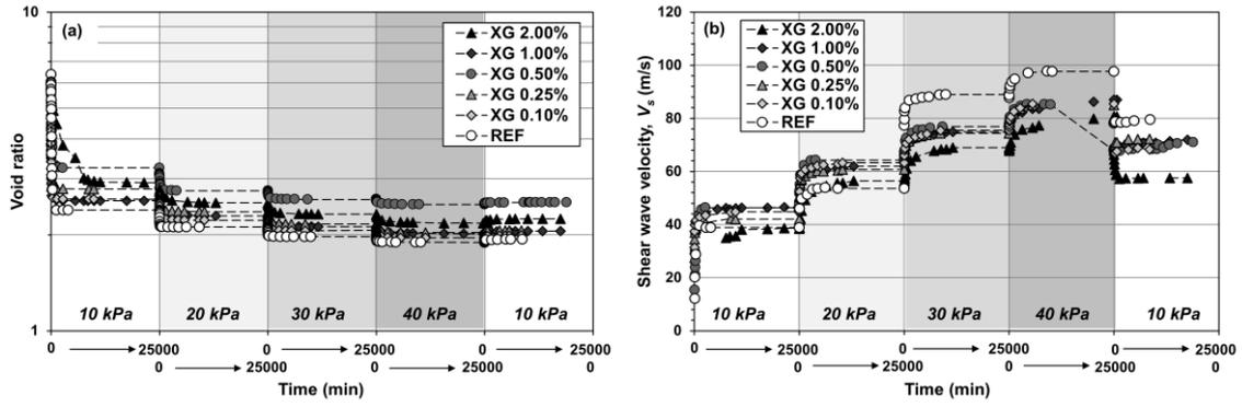
Fig. 4. Variation of (a) void ratio and (b) shear wave velocity during the laboratory consolidation test.
