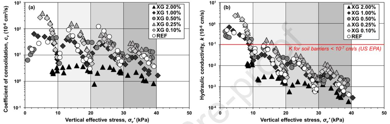
Fig. 8. Variation of (a) coefficient of consolidation and (b) hydraulic conductivity with vertical effective stress.
