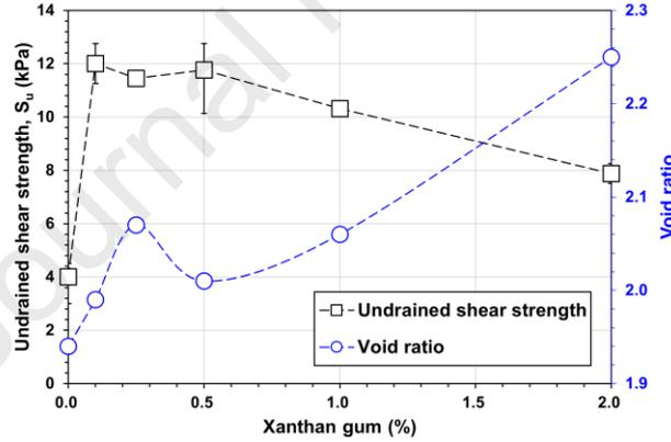
Fig. 5. Effect of xanthan gum treatment on undrained shear strength and void ratio.
