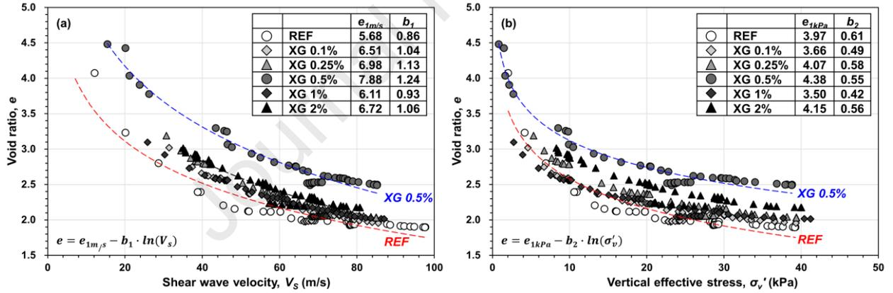
Fig. 7. Variation of void ratio with (a) shear wave velocity and (b) vertical effective stress.
